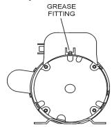
Figure 28. Grease Fittings Electric Motor
